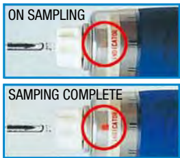
④ Take the sample. (Wait for 5 seconds after the indicator pops up.)
