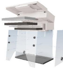
When the lower primary filter reaches saturation and fumes breakthrough they will be retained by the upper back-up filter. An inter-filter saturation alarm monitors the primary filter status and alarms upon breakthrough. The cabinet can continue to be used while waiting for replacement filters.
